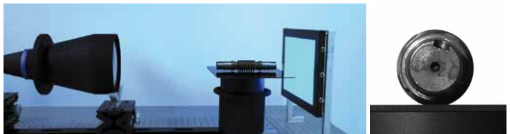
Image of a long object viewed along its field depth. The depth of field of OE telecentric lenses can hardly be achieved by other telecentric lenses.
